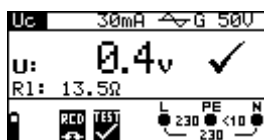
Figure 5.16: Example of contact voltage measurement results
