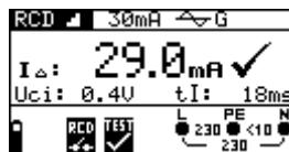
Figure 5.20: Example of trip-out current measurement result
