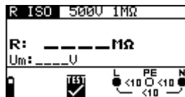
Figure 5.1: Insulation resistance measurement menu
