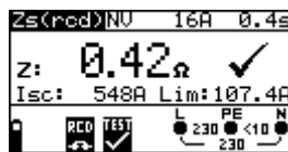
Figure 5.32: Example of fault loop impedance measurement results using trip-lock function
