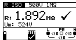
Figure 5.3: Example of insulation resistance measurement results
